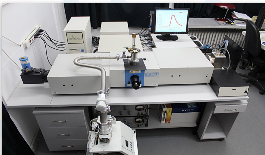
Spectrofluorimetru, model Fluorolog 3-22 (Horiba Jobin Yvon)
