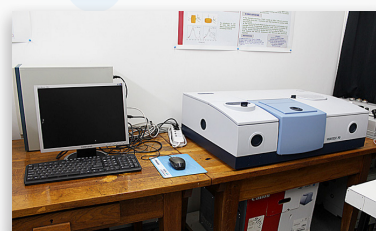
Spectrometru FTIR, model VERTEX 70 (Bruker Optics).
